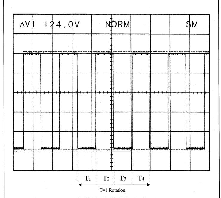
T=T1+T2+T3+T4 =(1 Rotation) T1=T2=T3=T4= $\frac{60}{4 \times \text{rpm}}$
