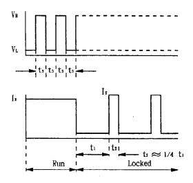
3rd wire signal Run : Square Wave Locked : V.
