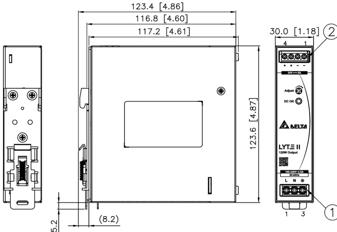
\*Unless otherwise specified tolerance of dimension are  $\pm 0.5$  mm
