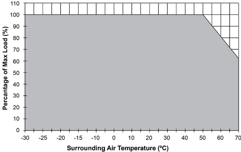
**Fig. 1 De-rating for Horizontal Mounting Orientation**
