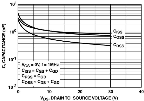
FIGURE 10. CAPACITANCE vs DRAIN TO SOURCE VOLTAGE
