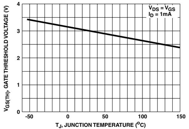
FIGURE 9. GATE THRESHOLD VOLTAGE vs JUNCTION TEMPERATURE
