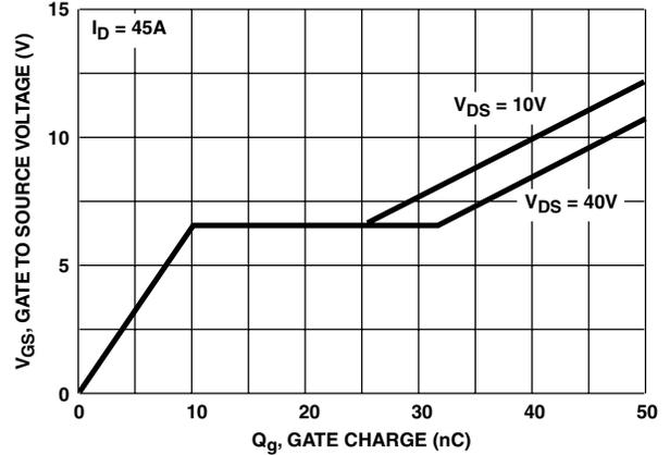
FIGURE 13. GATE TO SOURCE VOLTAGE vs GATE CHARGE
