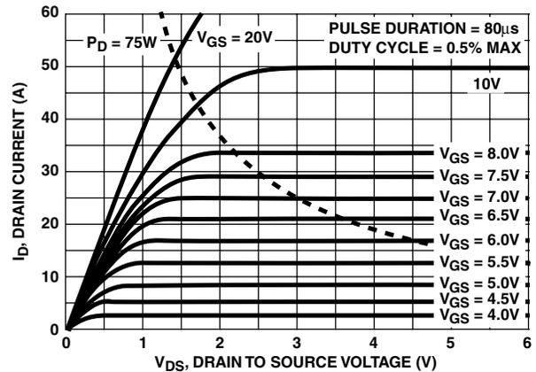
FIGURE 5. OUTPUT CHARACTERISTICS
