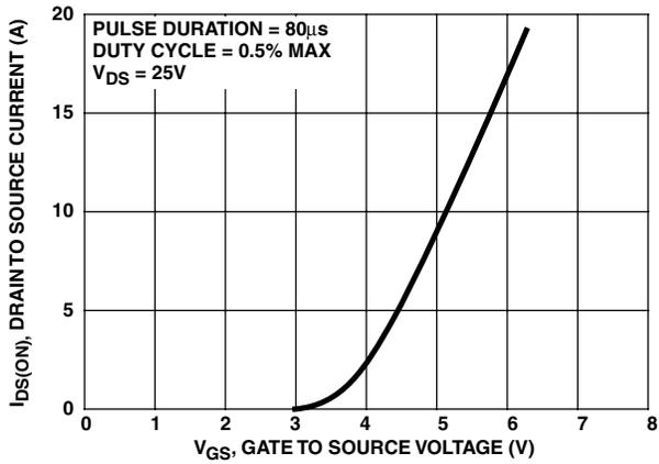
FIGURE 6. TRANSFER CHARACTERISTICS
