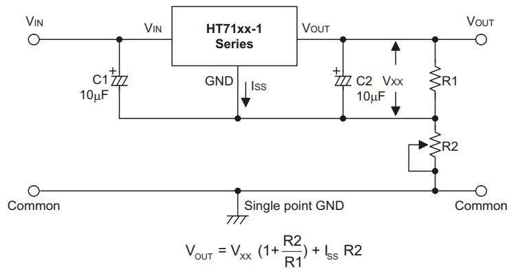
**Circuit for Increasing Output Voltage**
