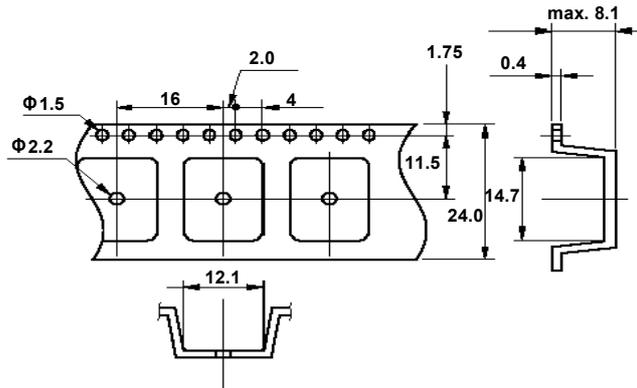
RELAY DIRECTION MARK AND TAPE CARRYING DIRECTION
