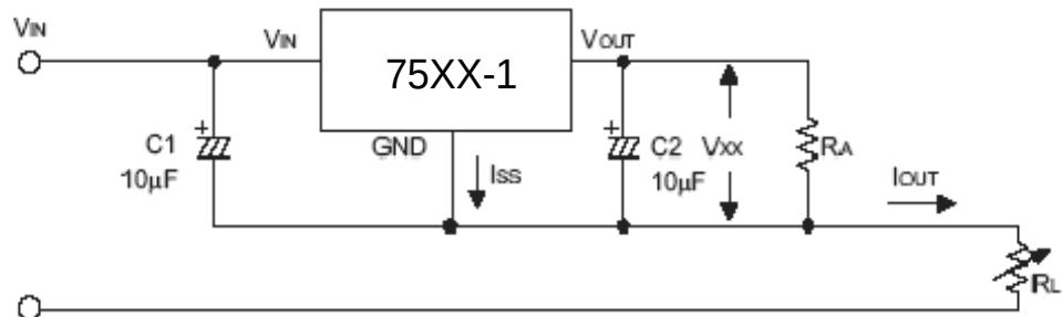
$$I_{OUT} = V_{XX}/R_X + I_{SS}$$
