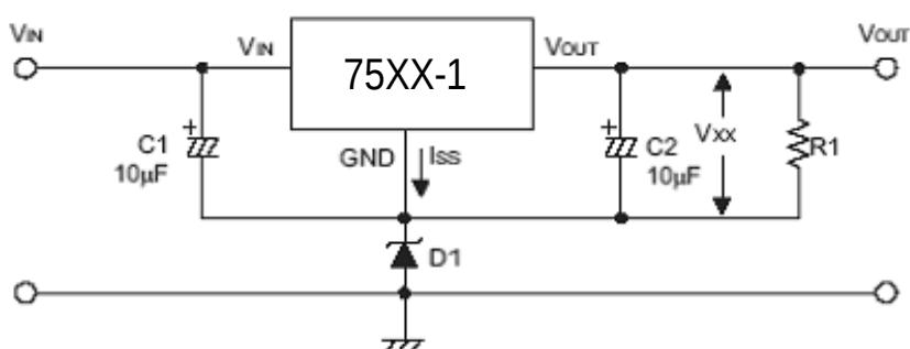
$$V_{OUT} = V_{xx} + V_{D1}$$
