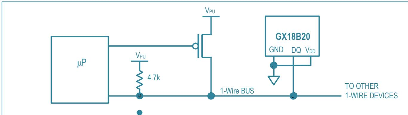
Figure 5. Powering the GX18B20 with an External Supply
