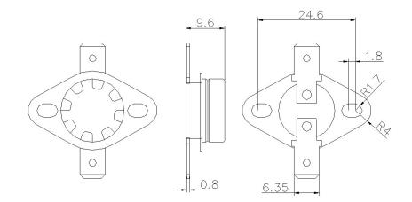
2.2 Terminal Strength: Terminals can bear tensile force of 80N and thrust of 70N.
