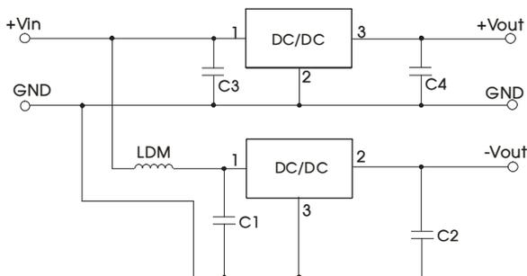
Fig. 3 Positive and negative output application circuit
