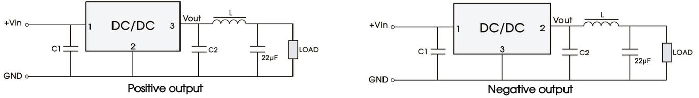
Fig. 4 "LC" output filter application
