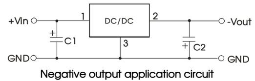
Fig. 2 Typical application circuit
