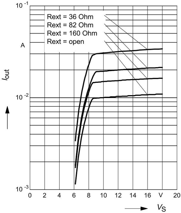
**Supply current versus supply voltage**
