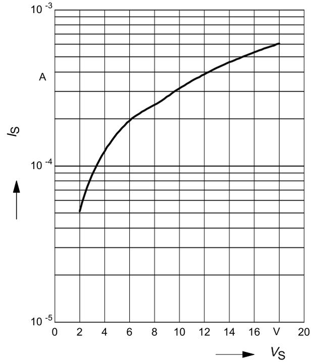
**Output current versus reference voltage**
