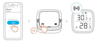
Tap "Add" on the main page of Zigbee Bridge on your eWeLink App, and long press the button on the device for 5s until the Zigbee signal icon (\*) flashes, now the device is entered the pairing mode and waiting to be added.
