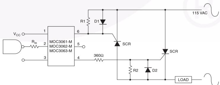
**Figure 11. Inverse-Parallel SCR Driver Circuit**
