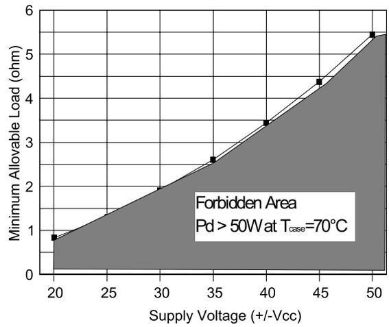
Figure 13: Modular Application Pd vs Vsupply (ref. fig. 7)
