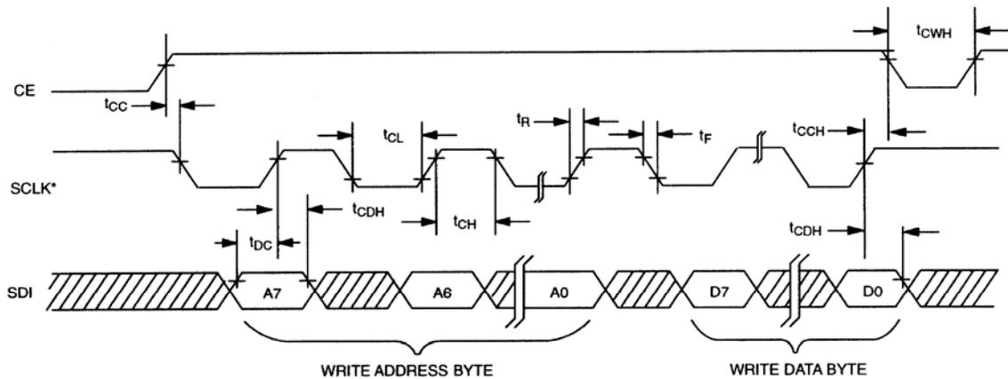
\*SCLK can be either polarity, timing shown for CPOL = 1.
