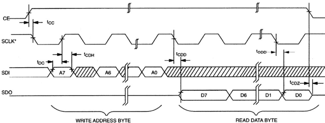
**TIMING DIAGRAM: SPI WRITE DATA TRANSFER** Figure 12
