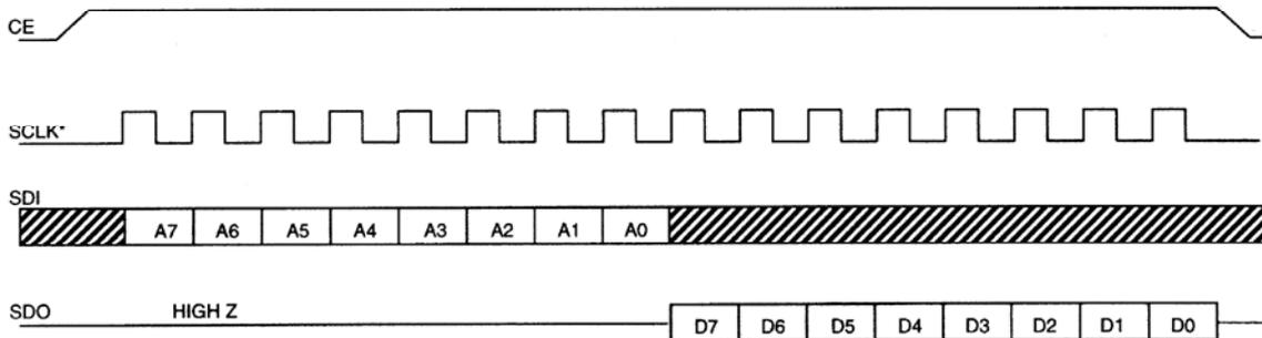
The address byte is always the first byte entered after CE is driven high. The most significant bit (A7) of this byte determines if a read or write will take place. If A7 is "0", one or more read cycles will occur. If A7 is "1", one or more write cycles will occur.
