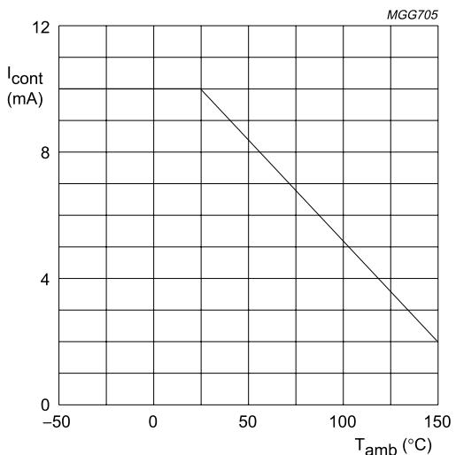
Fig.5 Maximum operating current for safe operation.
