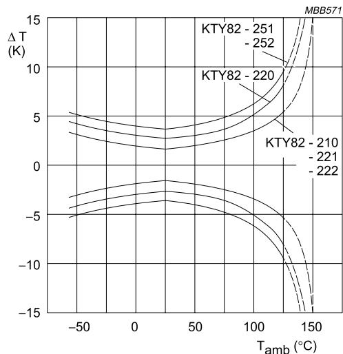
Fig.2 Maximum expected temperature error ( $\Delta T$ ).
