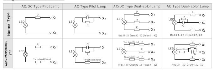
Note:1,AC/DC type pilot lamp is resistor step - down form; AC type pilot lamp is capacitor step - down form.
